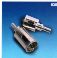
035 Diamond Core Drill With A Center Bit Dia: 30mm-85mm Diamond Grit: #40 Shank: Hexagon Or Round
