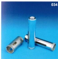
034 Diamond Core Drill With M14 or 5/8"-11 Thread Dia: 10-128mm Diamond Grit: #40
