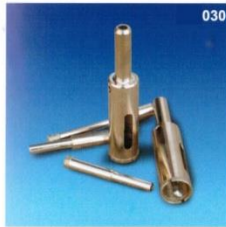
030 Diamond Core Drill With A Center Bit Dia: 6-128mm Diamond Grit: #100 Shank: Hexagon Or Round
